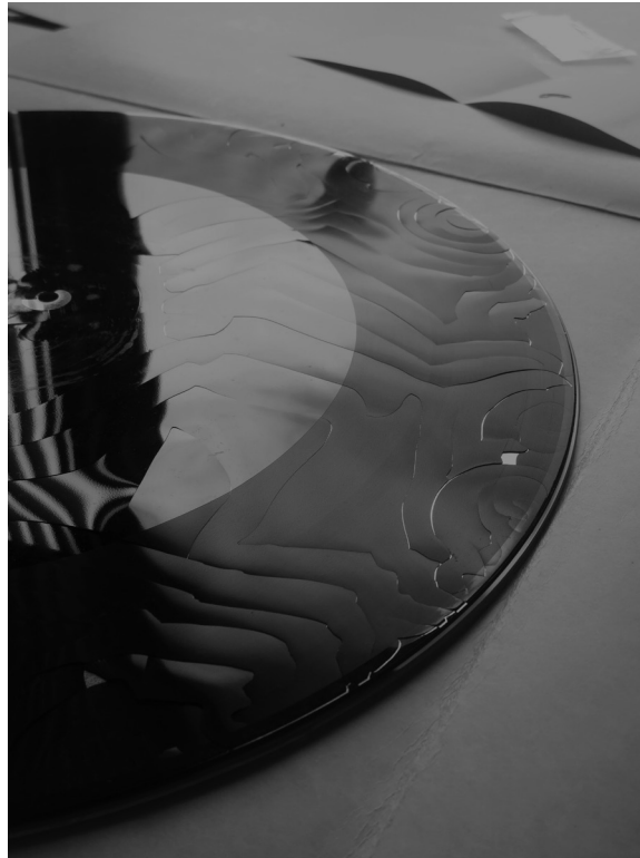
Figure 7: Lacquer lifting from aluminium base in irregular strips
