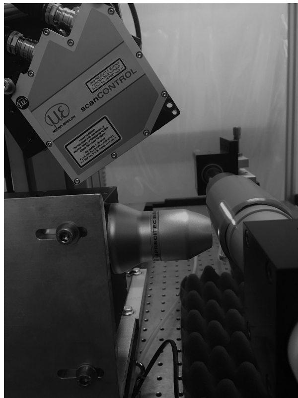
Figure 4: Confocal microscope scanning a wax cylinder
